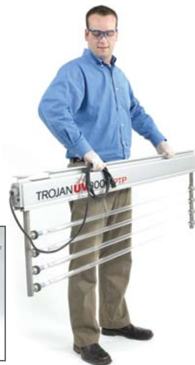
Lightweight, self-contained modules are operator-friendly and make routine maintenance quick and easy. Modules can be individually removed for periodic sleeve cleaning and lamp replacement after 12,000 hours (15 months). An optional, mobile cleaning rack simplifies maintenance procedures.
