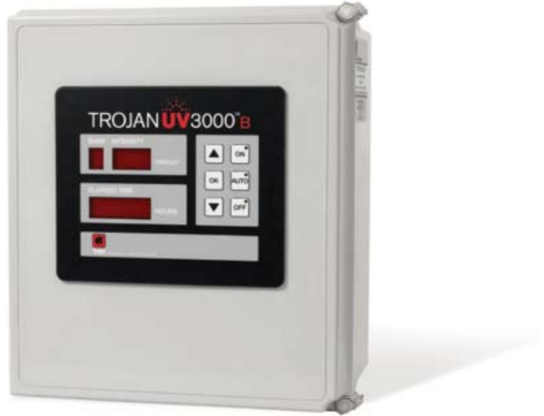
The System Control Center of the TrojanUV3000™B monitors lamp hours and uses a submerged UV sensor to feed accurate data on UV intensity for at-a-glance system status. The SCC also allows flow pacing to minimize operating and maintenance costs by turning banks on and off based on flow requirements
